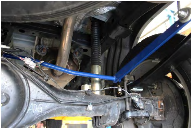
Figure 2 - Sway bar installation.
