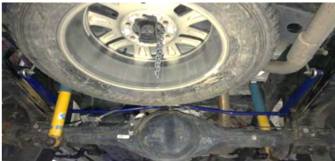
Figure 4 - Sway bar installation.
