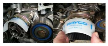
EZIGAUGE does not fit between the timing belt and the guide plate (where fitted) then loosen the guide plate retaining bolts and adjust the guide so the EZIGAUGE fits. **Only remove the EZIGAUGE after both bolts on the guide plate have been tightened.**
