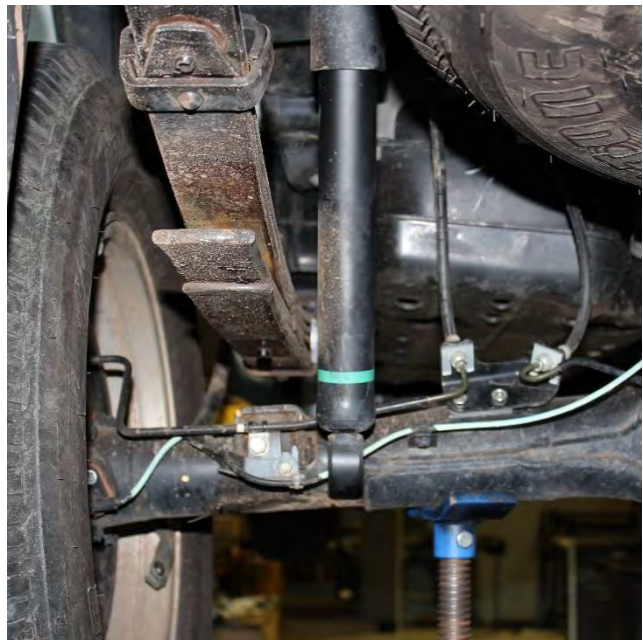
Picture 2: Installation of Raising Block
