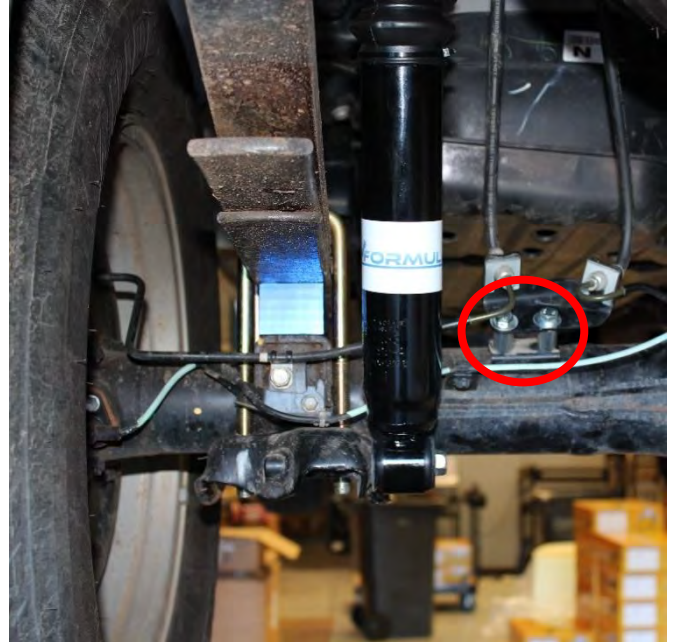
Picture 3: Installation of brake line spacer
