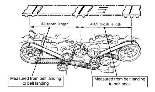
Due to manufacturing tolerances, these belt timing marks may not align perfectly with either the centre of the timing belt tooth or landing. Regardless, the correct count of tooth is as shown above and should be checked against actual timing belt with the crank reference mark being at the belt landing and the cam marks on tooth landing or tooth peak.
