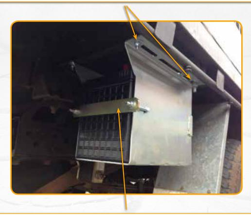
Sit battery into box and place battery hold down on, then tighten until battery is firmly in place.
