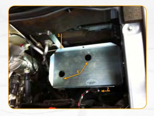
4. The two holes in the base of the tray have support legs which sit over two threaded bolts whitch are in the skirt. Fit 2 x 6mm nuts & washers on to these threads and tighten all nuts & bolts.
