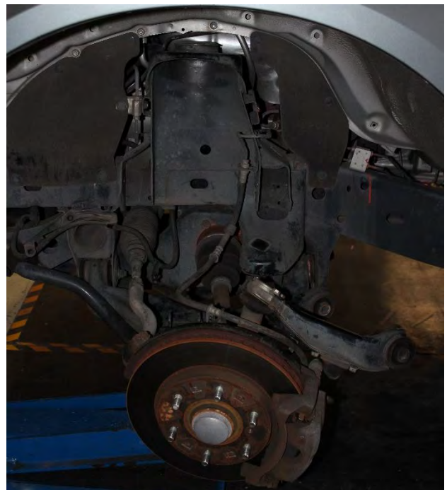
Picture 1: Front Strut Removal
