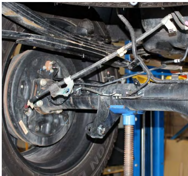
Picture 2: Raising Block Installation
