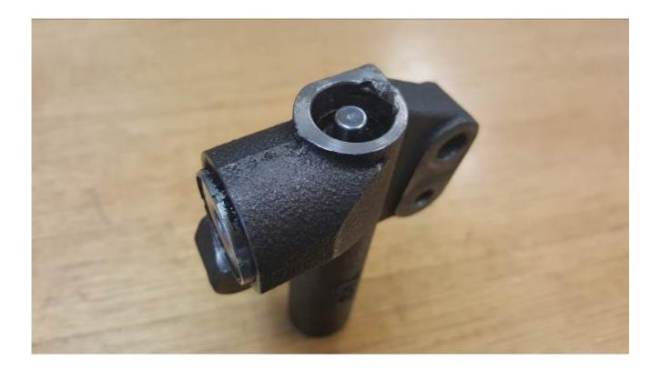
Evidence of HAT failures are actuator rods jammed in retracted position, and hammer marks around the HAT body where the tensioner assembly has come into contact with it. Example of which is shown above.
