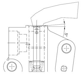
If these procedures and SST's are not used, the hydraulic actuator may operate in a range that will not provide the correct tension to the belt. This could cause a timing drive that either becomes noisy in operation or allows the drive to become unstable and lose timing or ultimately lead to failure of the timing drive.
