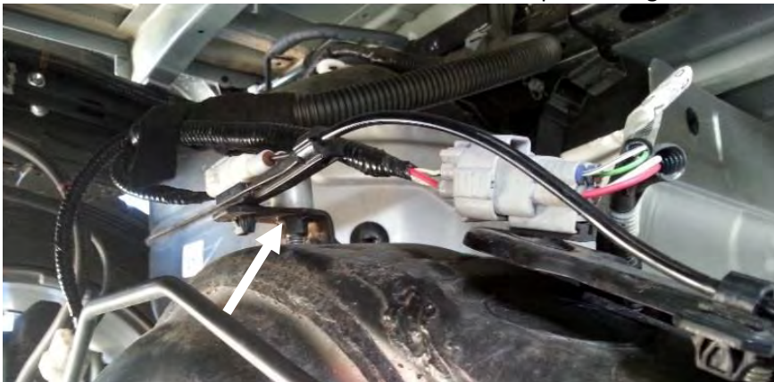
Picture 6: ABS cable mount position
